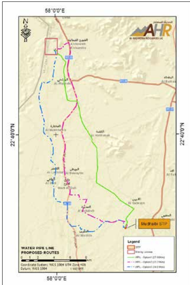
Figure 4: Water supply pipe line route from STP to project site
